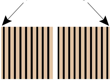
**Step 3**: With a caulking gun, apply a snaking line of adhesive to the back of the panel which will be installed on the left and then adhere it to the wall. Make sure to use a spirit level to make sure that it is straight.
