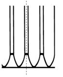
Multiple Ribbed panels: These panels will be cut at the base of a groove for the flutes to join together.
